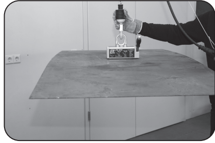
7. Run the lifting operation. Note that the shift of the lifting magnet must not be used as Hand guide
